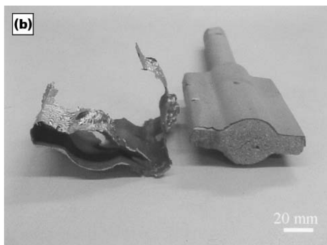
Fig. 13 Component 8 with thick alumina coating: (a) SEM micrograph showing the different regions of the component (from left to right, ceramic substrate, thick alumina coating, resin, aluminum resolidified and resin). The lighter region on the right (resin) results from surface charging and (b) aluminum layer easily removed from the shaft presenting an unaffected coating by the reaction test.
