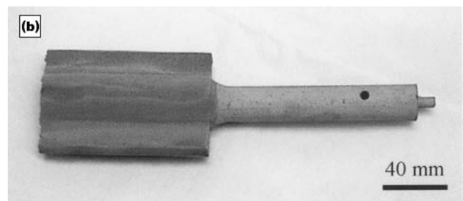
Fig. 4 Prototype for the reaction tests: (a) LOM prototype in the silicone mold and (b) coated ceramic component
